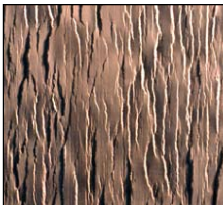
Overhead photograph showing extensional fault system in clay model
