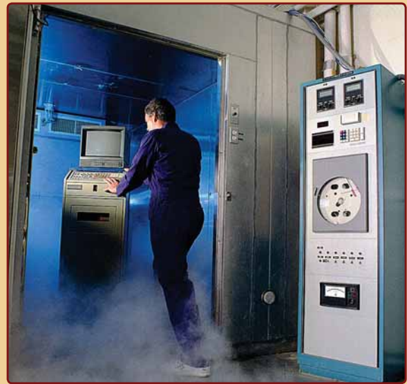
Equipment is placed in environmental chambers to evaluate performance in various temperature and humidity conditions.
