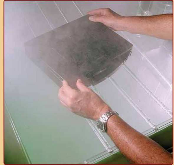
Equipment is evaluated for corrosion resistance of coatings and connections by exposure to simulated marine, coastal, and other corrosive environments.
