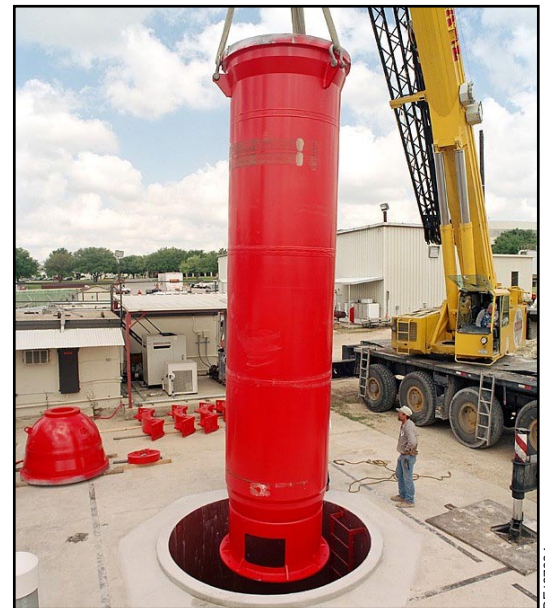
50-in ID, 24-ft long, 6,500-psi deep ocean test chamber at SwRI
