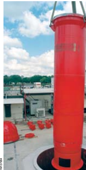
In April 2001 the Institute installed a new vertical chamber rated at 6,000 psig, 13,480 feet, 32°F. The chamber has hydraulic and electrical penetrations, and underwater cameras are available.
