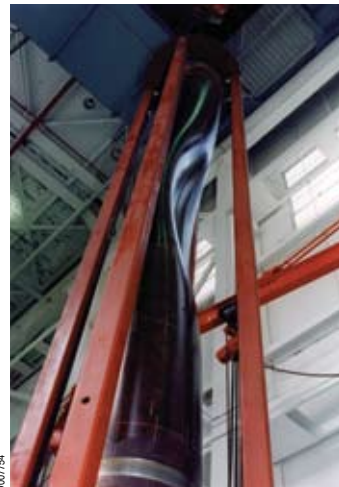
Large-diameter pipe casing after collapse test
