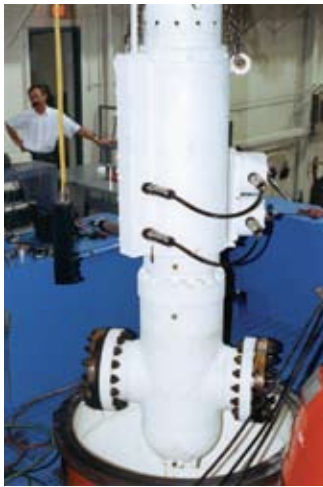
Subsea valve being placed in test chamber
