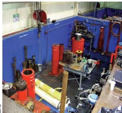
The main pressure laboratory houses more than 10 deep ocean pressure simulation chambers which are used for static, cyclic, and destruct testing.
