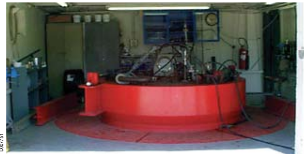
Test chamber 20 feet deep with 90-inch inside diameter
