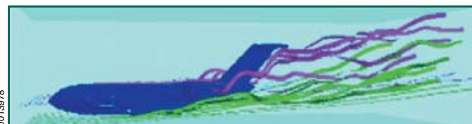
Aerodynamic simulation of airflow distribution around an aircraft during a pitching maneuver; wake region of aircraft is visualized by streamline ribbons
