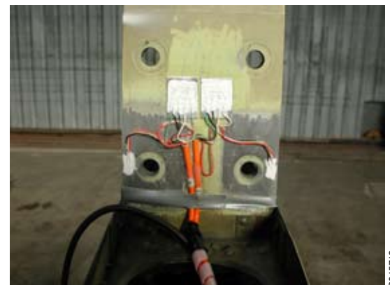
Typical strain gage installation
