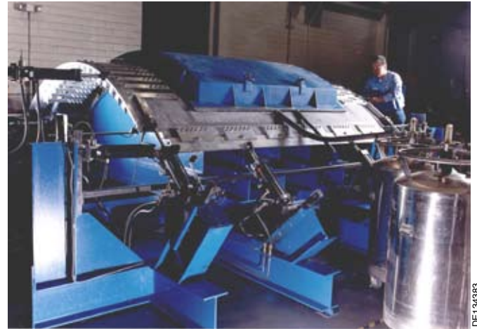
SwRI curved fuselage panel test facility being used to test a bonded repair with combined structural, pressure and thermally induced loads.
