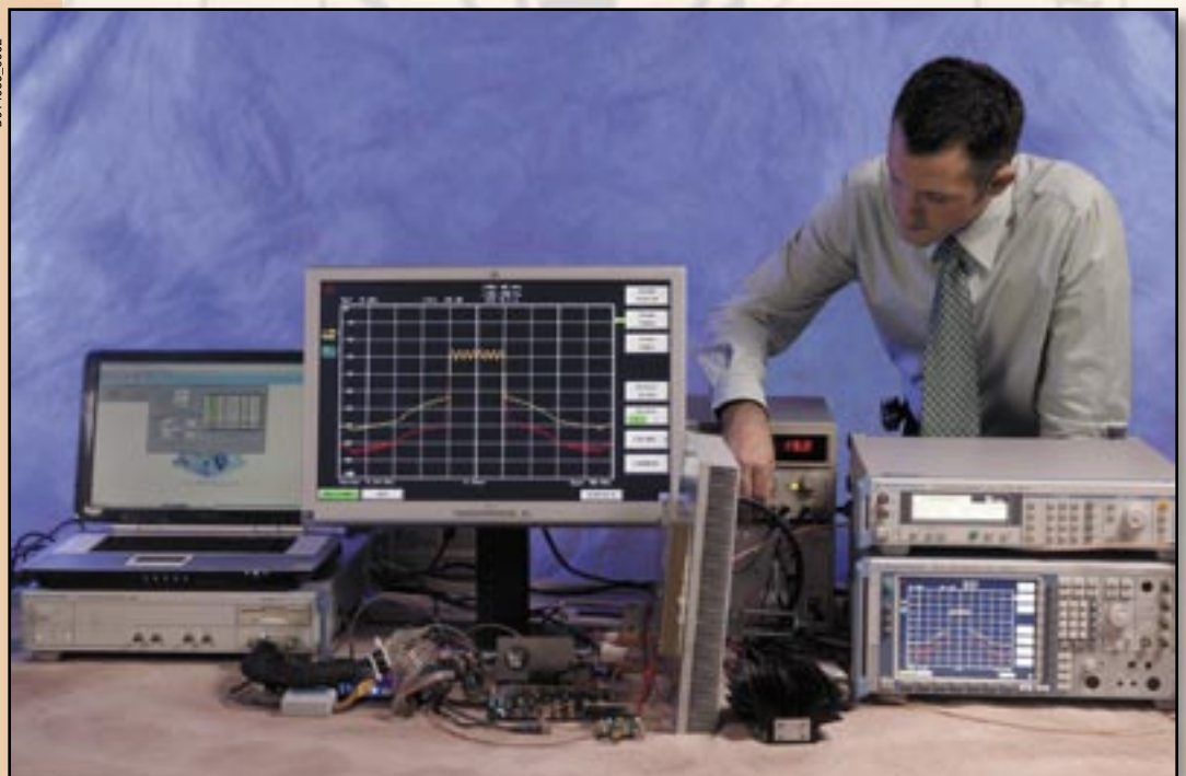
SwRI engineers develop a digital predistortion hardware-in-the-loop demonstration system.
