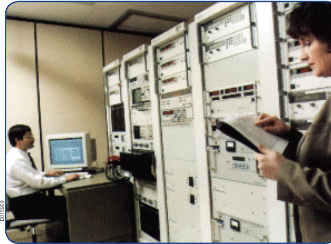
SwRI has developed hardware and test programs for a number of large, ground-based automatic test systems. This depot power supply tester was developed for F-15 aircraft support equipment.
